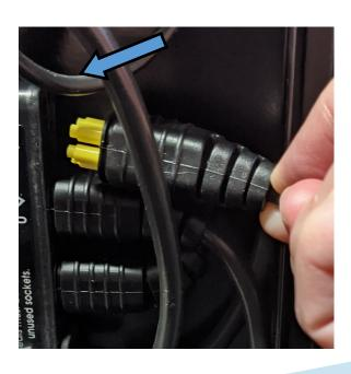
4. Plug the RNet cable into the APR
