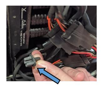
3. Plug the RNet cable into the RNet bus on the back of the chair. Note if you are installing an IOM at the same time you will plug in 2 RNet cables that will run parallel.
