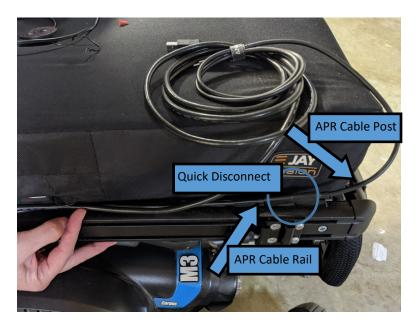
7. Plug the USBC cable from the APR into a USBC power port on a supported device.
