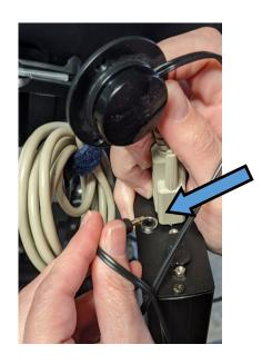
8. Plug the single screw end of the USBC cable into the ADT. Screw in the cable.
