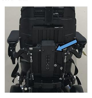
2. Remove the waterproof plug on the RNet bus bar  $\,$
