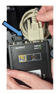
7. Plug the other end of the 9Pin cable into the ADT. Screw in the 9Pin cable.
