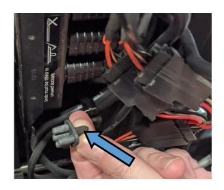
3. Plug the RNet cable into the RNet bus on the back of the chair. Replace the back panel.
