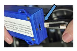
9. Plug the USBC cable into a supported device.
