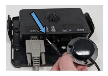
4. Plug the single screw USBC cable into the ADT. Screw in the cable.
