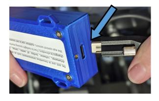
6. Plug the USBC cable into a supported device
