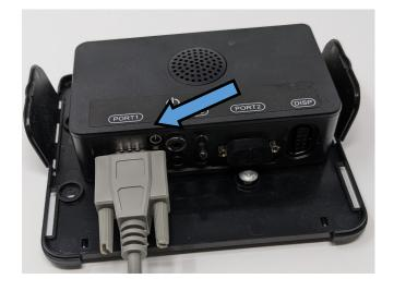
2. Plug the other end of the 9Pin cable into the ADT. Screw in the 9Pin cable.
